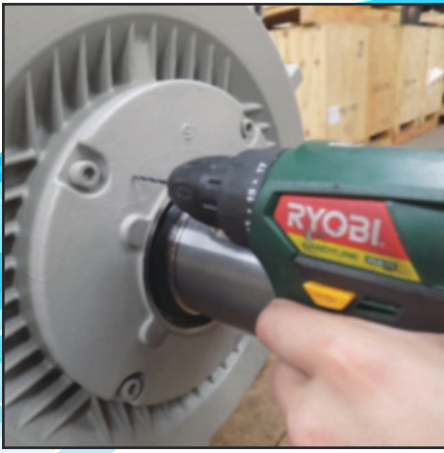
9) Drill hole with 2.5mm Steel drill bit.
