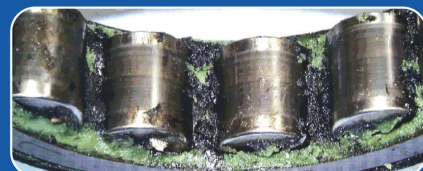
Eddy Currents Damaging Bearing Grease - Increasing Service Intervals.
